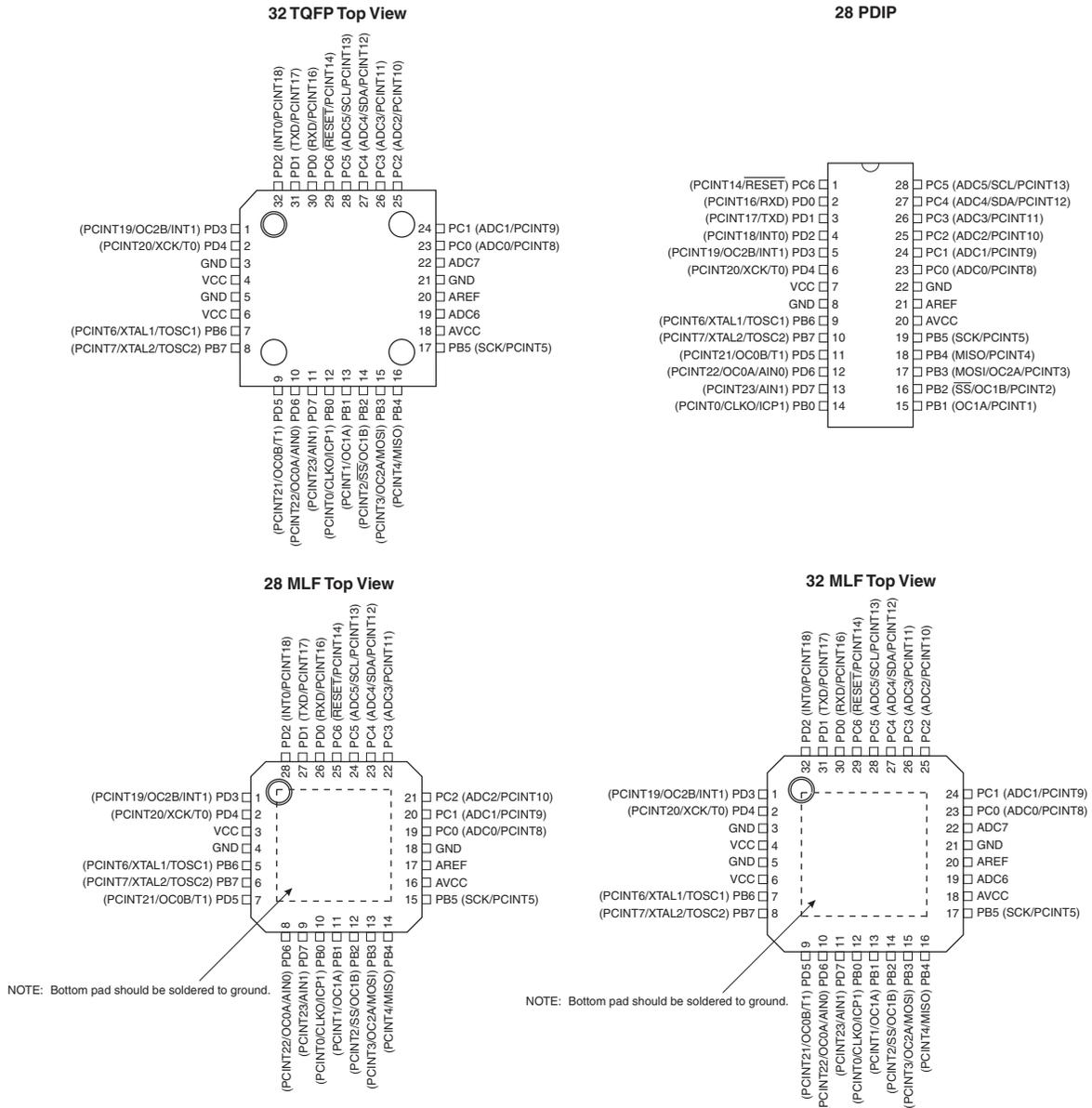
Table 1-1. 32UFPGA - Pinout ATmega48A/48PA/88A/88PA/168A/168PA
